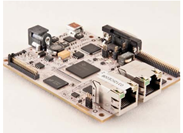
The AM3359 industrial communication engine (ICE) is a cost optimized pocket-size development board for I/O devices and sensors. Photo: TI
