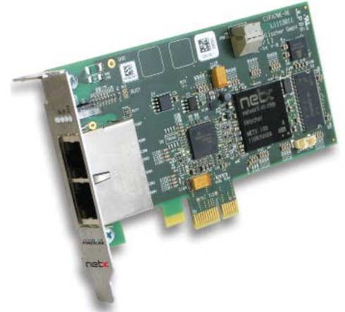
The cifX 70E by Hilscher makes POWERLINK available for Low Profile PCI Express
