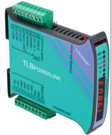
The compact as well as universal weighing instrument TLBPOWERLINK by Laumas features a POWERLINK port for fast data exchange.
