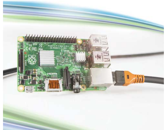
Kalycito has implemented POWERLINK on a Raspberry Pi2 with Linux.
