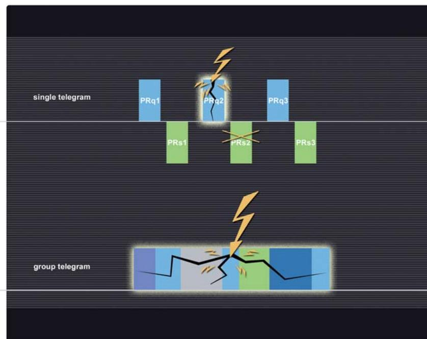
Figure: Electromagnetic interference merely results in destroyed single telegrams in POWERLINK networks, while the complete cycle is affected in group telegrams.
