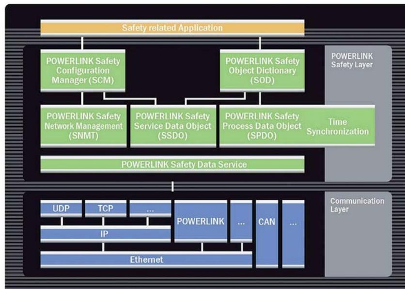
Figure: Diagram of the POWERLINK Safety Layer
