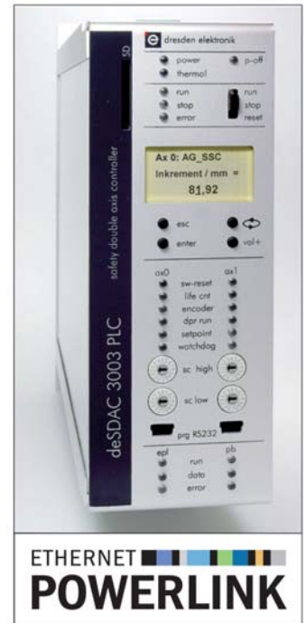
Figure: The deSDAC 3003 PLC drive controller features a POWERLINK interface
