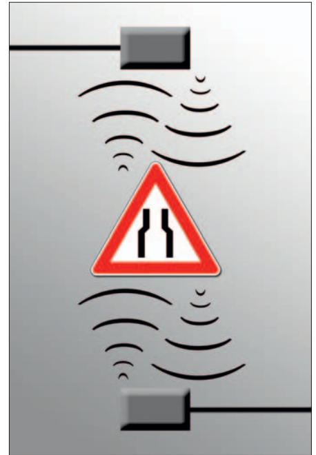
Figure 1: Wireless data transfer creates additional delay times. The decision for or against using WLAN always depends on the required real-time determinism.
