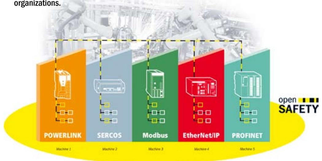
openSAFETY enables a unified safety standard for complete plants, regardless of the control system manufacturer and the fieldbus standard
