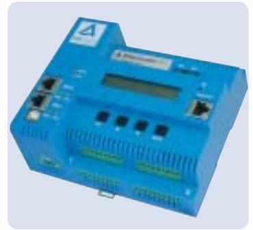
analyze the EPL network. The Ethercontrol I/O modules feature different combinations of binary digital, analog or encoder inputs or outputs, which make them ideal complementary components e.g. for existing drive controllers.
