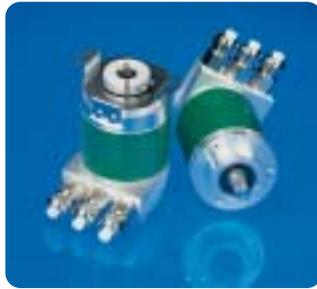
integrated dual port hub. Diagnostic LEDs indicate Powerlink device status information and Ethernet network diagnostics (link, collision, receive). A network address is assigned to an encoder by setting its device IP address using two turn switches on its interface unit. The encoders also accept control commands for configuration, either as TCP/IP frames or via an integrated web server.
