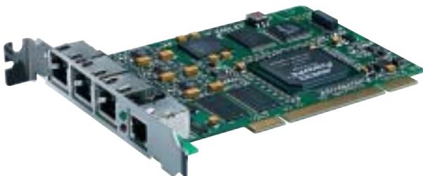
PCB. The interface is suited for communication with one or two EPL networks, depending on the required level of performance. It is designed for Windows 2000/XP (embedded) and Linux;
